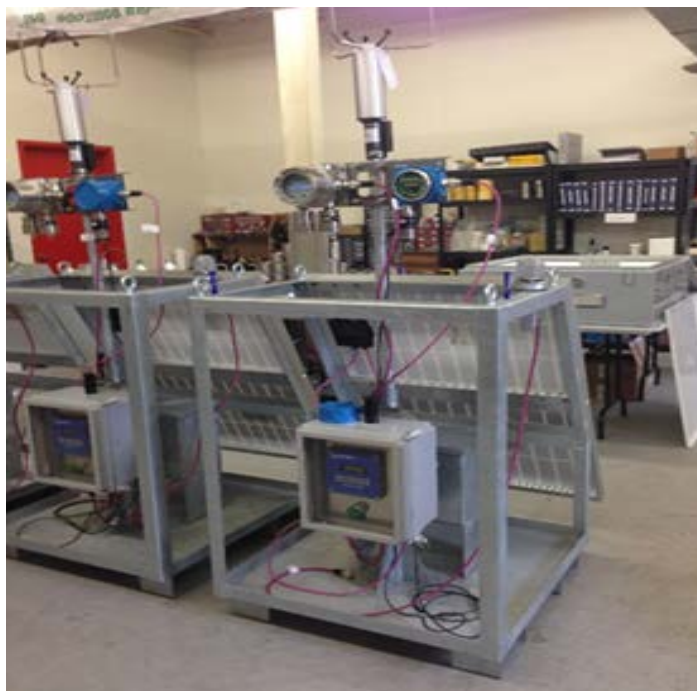
Weatherproof enclosure with solar panel and meteorological sensors.
